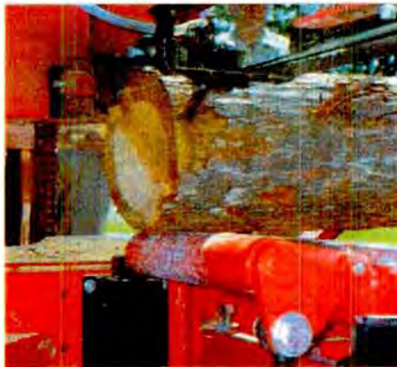
The log-tapering devices consist of two rolls powered by hydraulic cylinders, located on either end of the frame bed.
